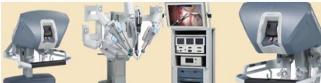
Figure 34: da Vinci Surgical System Si, integrated robotic system with working console, side cart and control unit (Intuitive Surgical)
