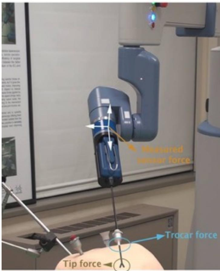
Figure 38: Telelap ALF-X unit for measuring trocar force (Sofar)
